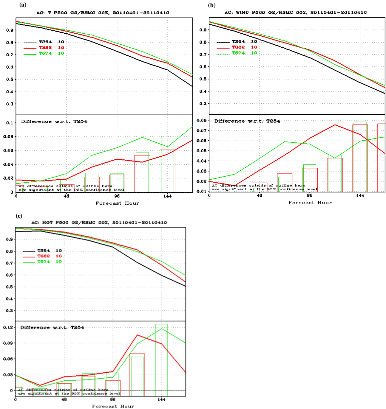
Figure 28: Anomaly Correlation (AC) at 500hPa over RSMC region (upper part) and difference of Mean (AC) w.r.to T254L64 and its statistical significance (lower part) for (a) Temperature, (b) Vector Wind, and (c) Geo-Potential Height.
